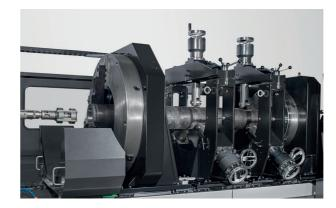
The **rotation device** prevents axis misalignment and guarantees a better bore geometry. The **steady rests** (standard from 6 m) are easily to set up.
