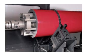
The **universal V-type chain fixture** is simple to adjust and has a large diameter range up to 1'000 mm.
