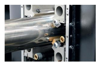
The **stone holder system** allows the stones to be mounted with one screw with only 1/2 turn, which enables a short changeover time.
