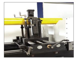
Fixturing has been developed that reduces set-up time and is easy to move on rails. No air is required.
