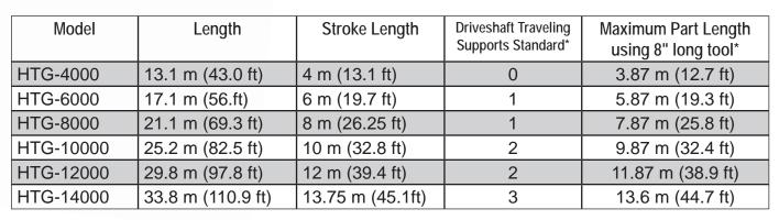
\*Optional driveshaft traveling support may be added depending on application. Stroke length of machine is reduced by 244 mm (9.6 in.) when a third support is added.
