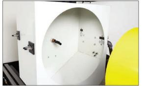
The interlocked rear splash guard incorporates parts present sensors as well as moveable nozzle to deliver honing oil/coolant where needed. SPECIFICATIONS: SPINDLE SPEED: 0 - 300 RPM
